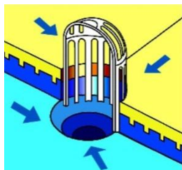
Roof Water Outlet
